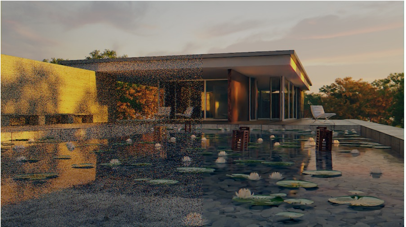
Fig. 267: Render before and after denoising, with a very low number of samples as input. As more samples are used, the denoiser will be able to better preserve detail.
