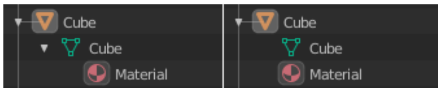
Fig. 520: A material linked to Object Data (left) and Object (right).
