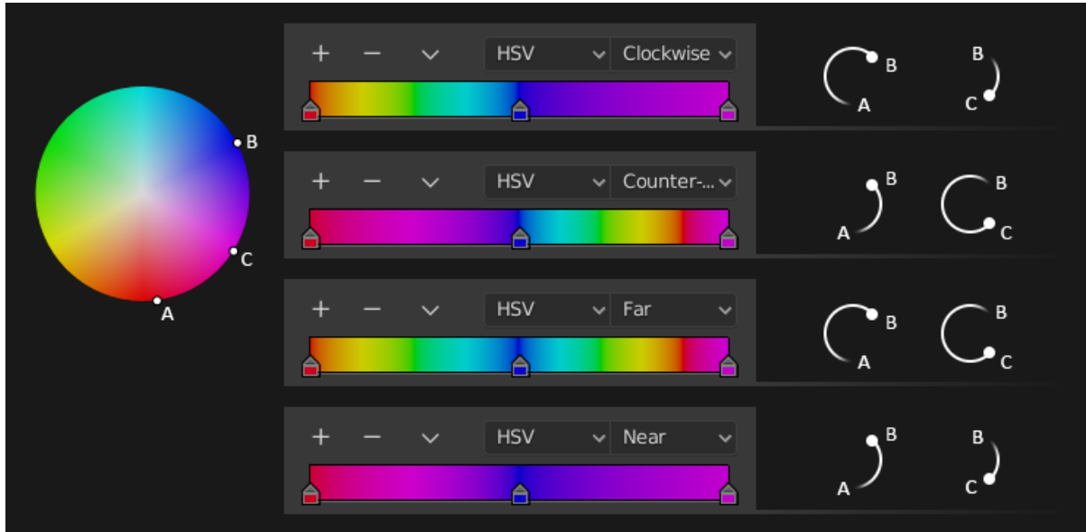
Fig. 44: HSV and HSL interpolation options.
