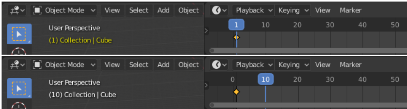
Fig. 1562: Top: Current frame is a keyframe for Cube. Bottom: Current frame isn't a keyframe.
